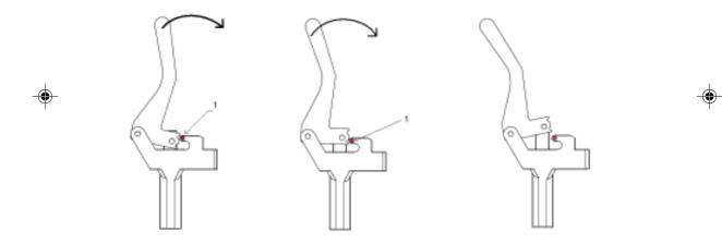
To lock the brake lever in Position 1, or Position 2 pull it to the required position and press the red button (marked no 1). In order to release the brake, pull the lever harder to enable the automatic release of the lock.
